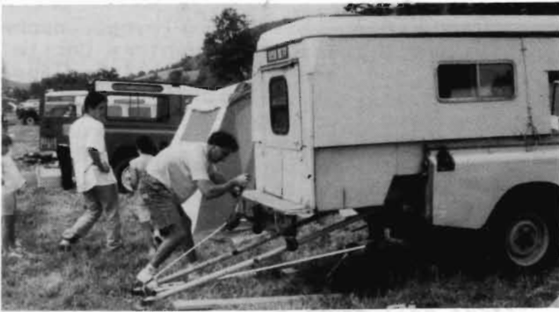
Hand winch cable enhanced back to tow-ball
