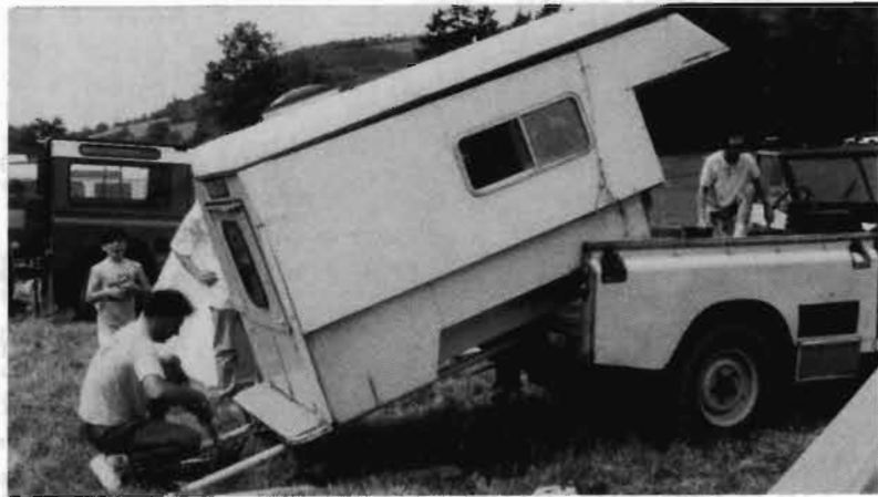
Hand winch cable enhanced back to tow-ball
